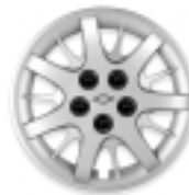
16" steel wheel with bolt-on wheel covers — standard on Monte Carlo LS.
